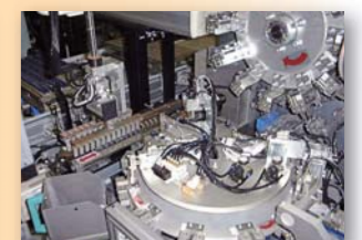
Condenser assembly system
